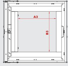
Clearance dimensions: A3 x B3. assembly dimension A1 x B1.
