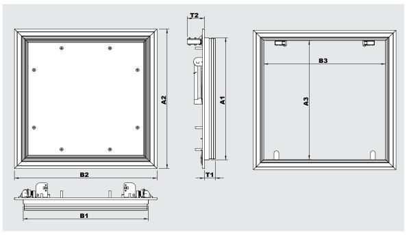
Clearance dimensions: A3 – 32 mm x B3 Cutting dimension: mounting dimension A1 + 5-10 mm x B1 + 5-10 mm
