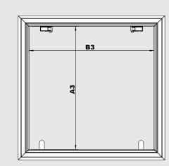
Clearance dimensions: A3 – 32 mm x B3 Cutting dimension: mounting dimension A1 + 5-10 mm x B1 + 5-10 mm
