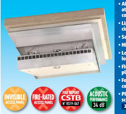
120-minute fire-rated ceiling access hatches are designed to be installed in self-contained fire protection false ceilings. One of the requirements is that the «fire load is only on the room side», and the fire resistance classification is El 120.
